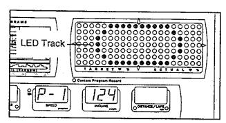
a "P-1" will appear in the SPEED display and the current weight setting will begin to flash in the INCLINE display. The LED track will also be lit. Note: When you are familiar with the console, you may go directly to step 6 if desired. The first time you use the console, please follow all steps.
